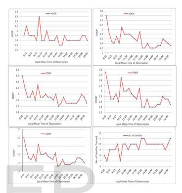
**Fig. 12**: Post-observation DOPs [GDOP, PDOP, HDOP, VDOP and TDOP] values and available satellites
