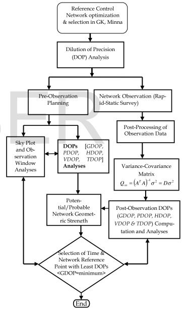
Fig. 5: GPS Ground Control Reference Network Optimization and Selection Algorithm for Gidan Kwano Area of Minna, Nigeria
