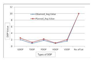
Fig 14: Comparison of the Mean DOPs from Pre- and Post Observations
