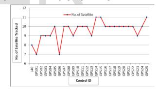
Fig. 9: Number of satellites tracked at control stations during Observations
